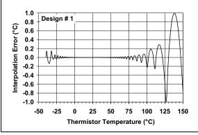
FIGURE 9: Piece-wise Linear Interpolation Error, Design # 1.
