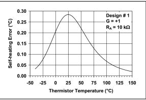
FIGURE 5: Thermistor Self-heating Error.
