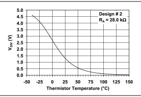
FIGURE 10: Voltage Divider Output.
