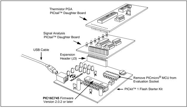
FIGURE A-3: Board Connections.
