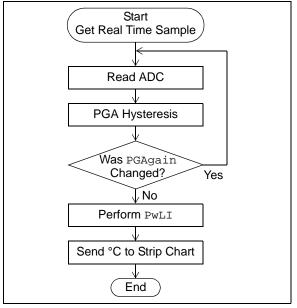
FIGURE 15: Flowchart for Second Design.
