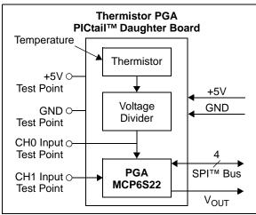
**FIGURE A-1:** Thermistor PGA PICtail<sup>™</sup> Daughter Board Block Diagram.
