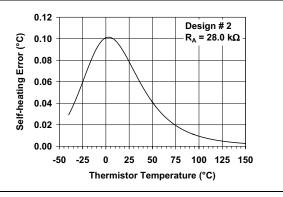
FIGURE 11: Thermistor Self-heating Error.
