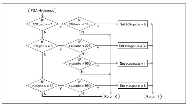
FIGURE 16: Flowchart for Second Design's PGA Hysteresis Subroutine.
