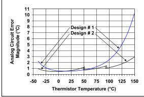
FIGURE 20: Analog Circuit Error Comparison.
