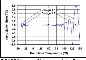
FIGURE 21: Digital Interpolation Error Comparison.
