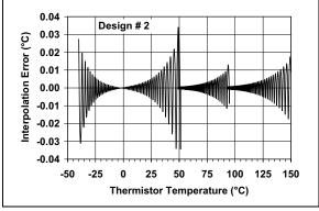
FIGURE 17: Piece-wise Linear Interpolation Error, Design # 2.
